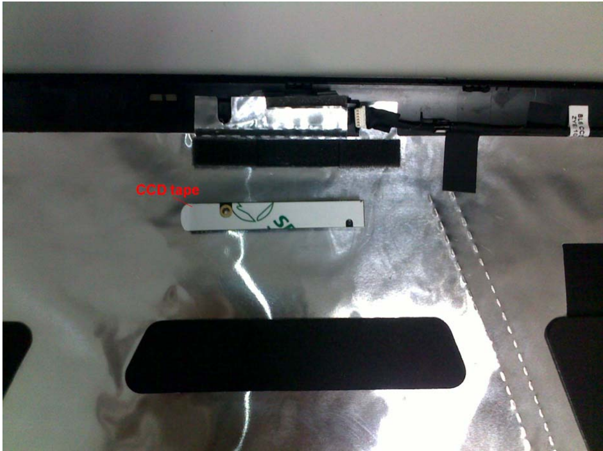
Figure 4-20-3 Camera Module before installing
