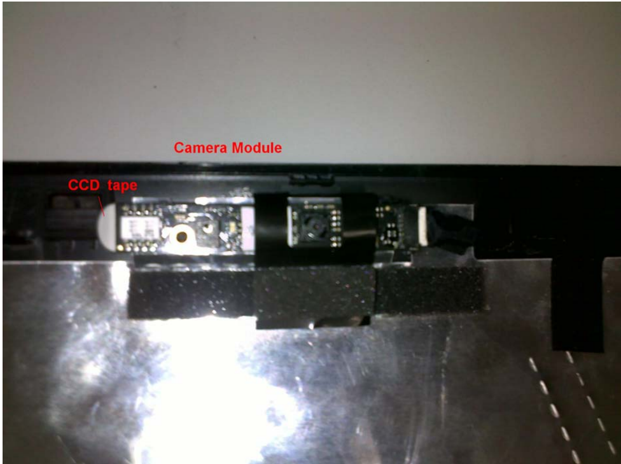
Figure 4-20-4 Camera Module after installing
